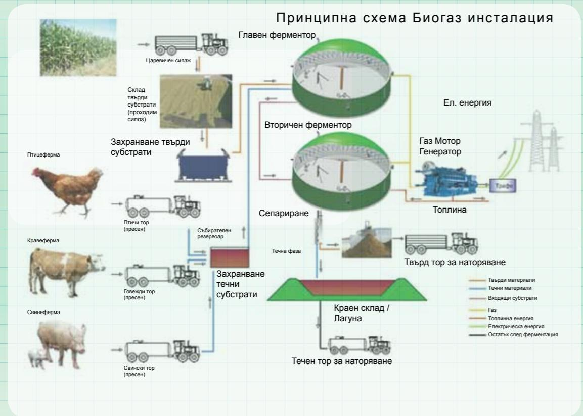
**BIONA** Schematic biogas plant
